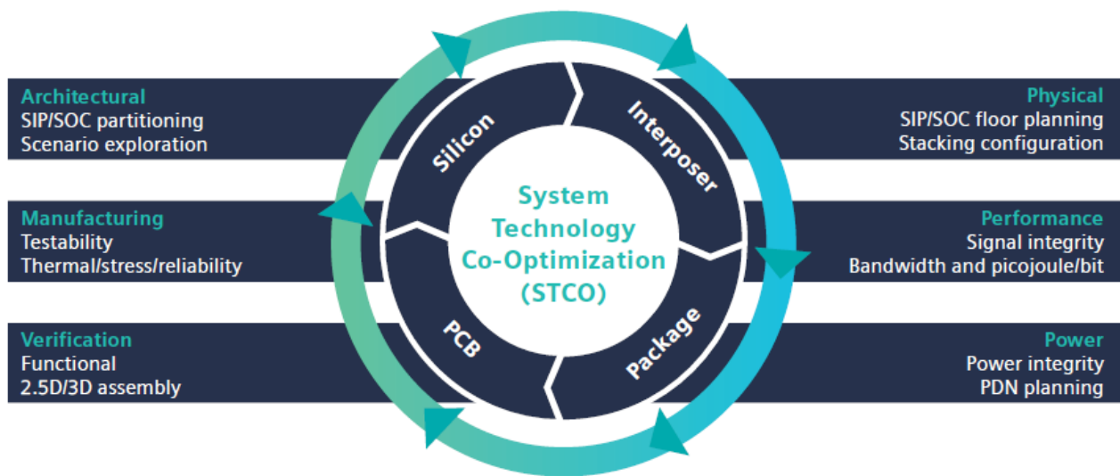
Figure 5: STCO enables co-design and optimization across the entire package assembly, from the silicon die to the PCB motherboard (© SIEMENS EDA)
